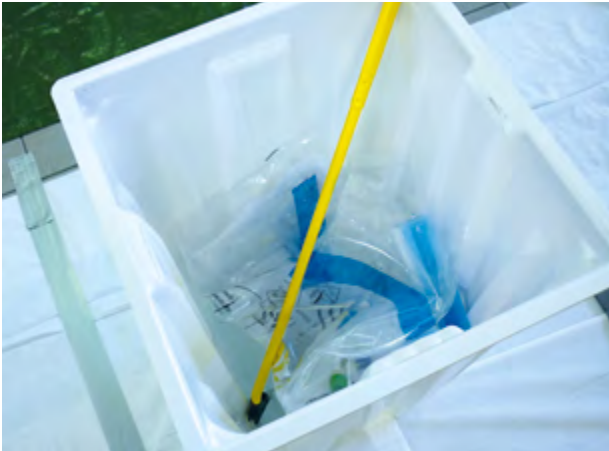
Fig. 3: Example of a disinfectant bath: Sample bags can be dipped in decontamination solution.
