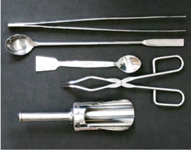
Fig. 9: Suitable sampling materials for solids (from bottom to top): scoop, crucible tongs, small spoon spatula, large spoon spatula, tweezers
