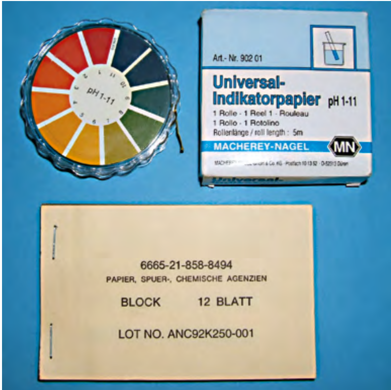
Fig. 17: Universal indicator paper, pH range 1-11
