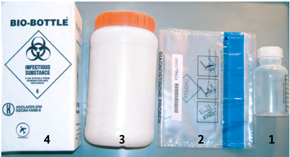
Fig. 18: Example packaging in line with P 620 (ADR): Sample container (1) = primary container, PE bag (2), secondary packaging (3) and external packaging (4) (carton)
