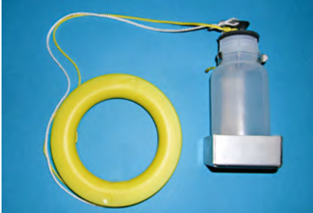
Fig. 11: Water sampling device for removing water from a specific depth
