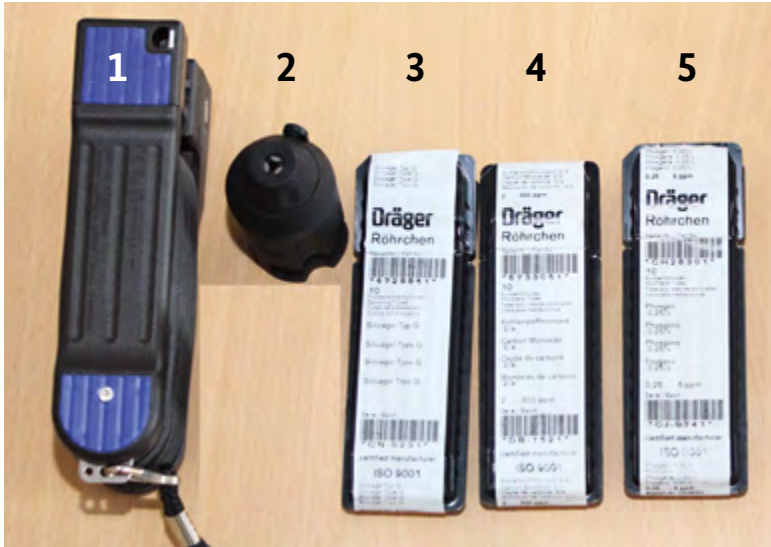
Fig. 14: Government-issue CBRN equipment with hand pump (1) and tube opener (2), silica gel sorbent tube (3) and direct-reading short-term measuring tube for carbon monoxide (4) and phosgene (5)
