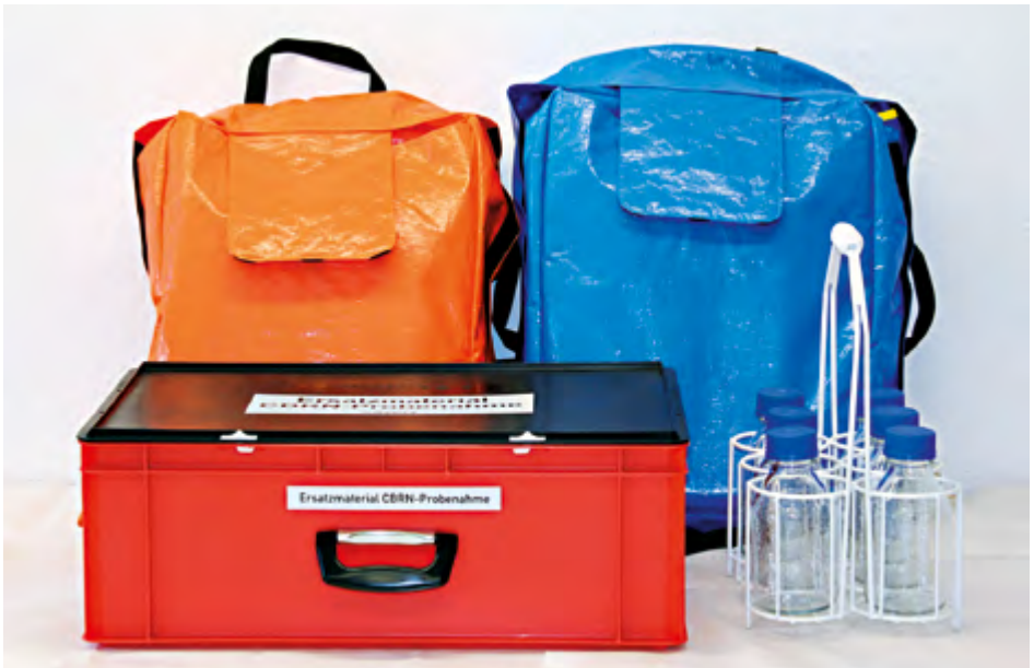
Fig. 6: Packs from the government-issue CBRN sampling equipment
